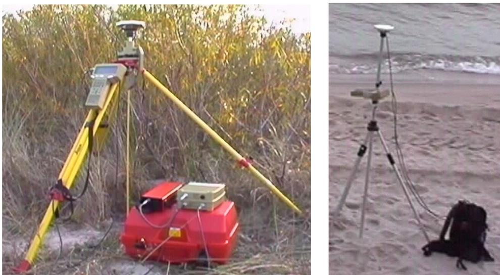
Fig.1. Leica SR-9500 GPS Total Station system
